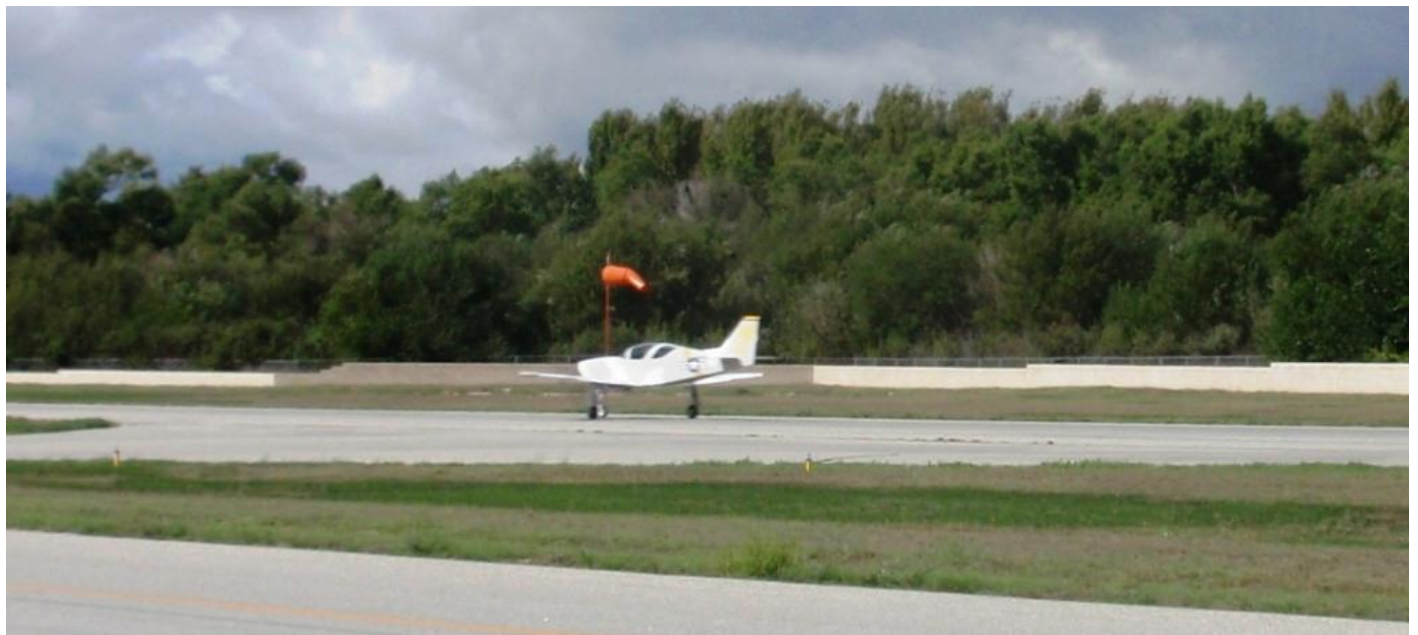
This high horsepower plane has small wings, and uses a lot of runway to get off the ground
