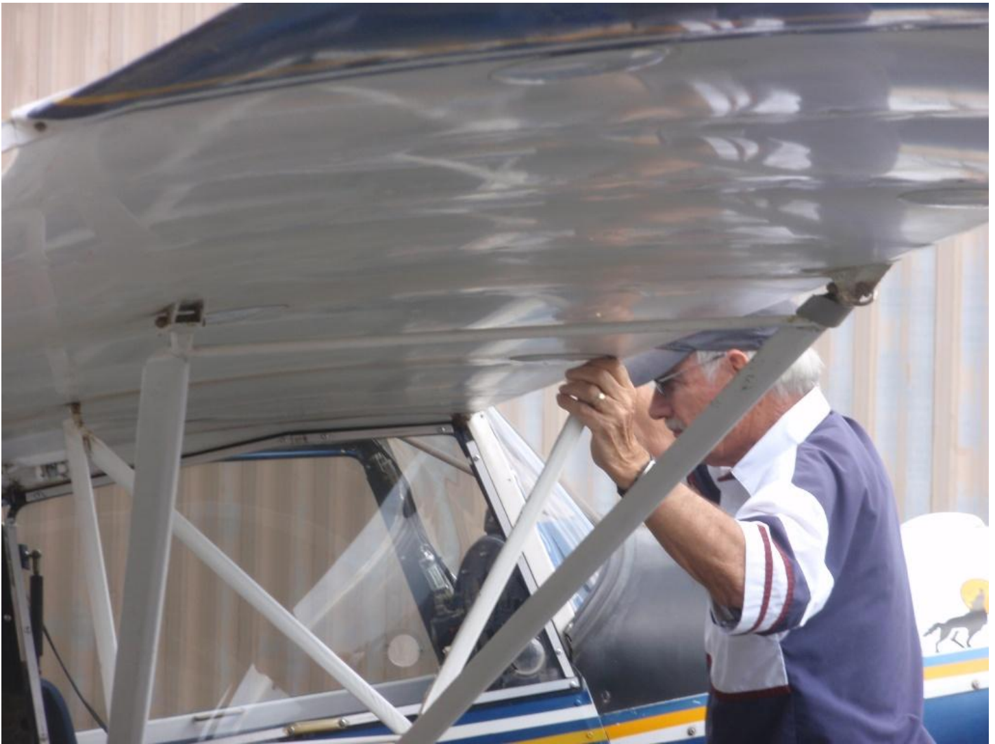
John removed the locking pin and started to swing the wing back on the hinge at the rear of the wing
